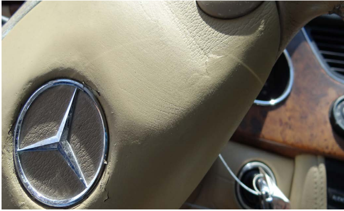
Repair of previously deployed front airbag module.
