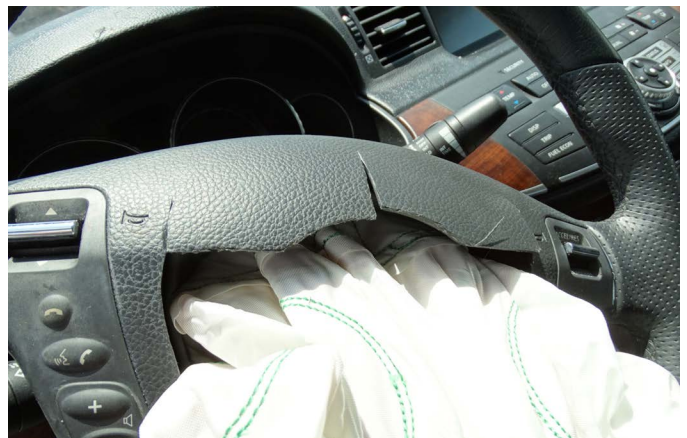
Front airbag module was cut open and airbag pulled out.
