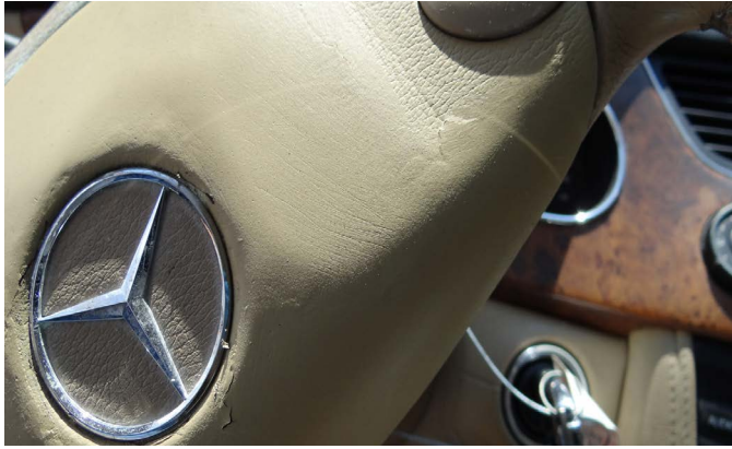
Repair of previously deployed front airbag module.
