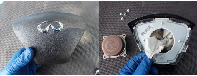
Front airbag module (left). Ignitor removed and previously deployed air bag found (right).
